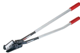
Model CU-25LH Part No. 0X-1528 Extra long handle cutter. Replaceable blades. Cuts strap through 2" x 0.050" (50.8 x 1.27 mm). Shipping weight: 8 lbs. (3.6 kg)
