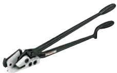
Model CU-25 Part No. 005740 For strap removal or cutting strap to length. Replaceable blades. Cuts strap through 2" x 0.050" (50.8 x 1.27 mm). Shipping weight: 8 lbs. (3.6 kg)
