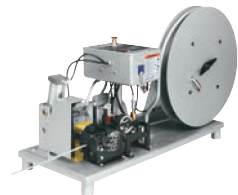
DPCL Cuts strapping automatically up to 100 ft. in length.
