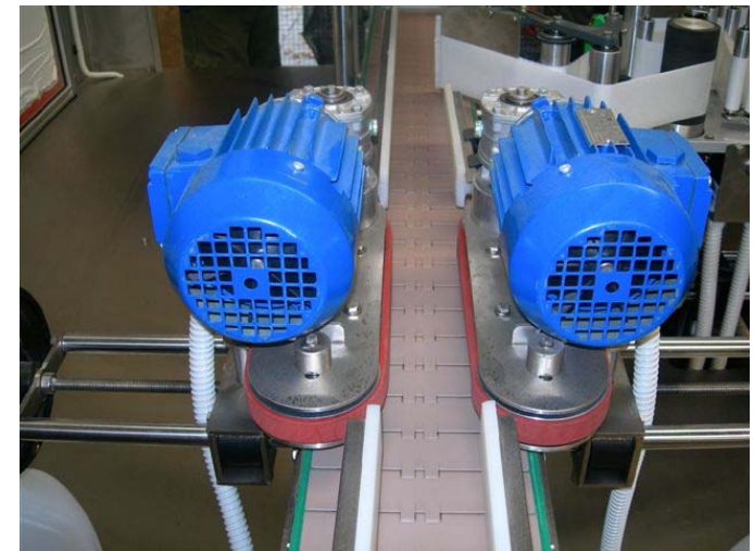
Equipped Standard with In Feed Spacing Drive Belts
