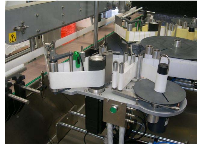
Dual Applicators- System Switches Between Label Applicators to Ensure Increased Uptime!
